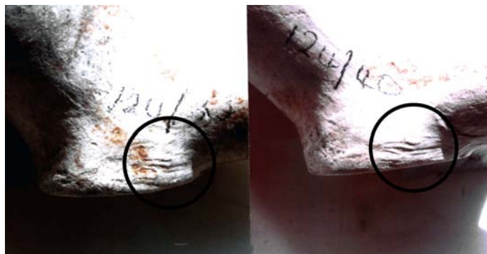
Seventeenth-century pipes from Pontefract Castle showing matching mould flaws (circled). Photo S. D. White.
