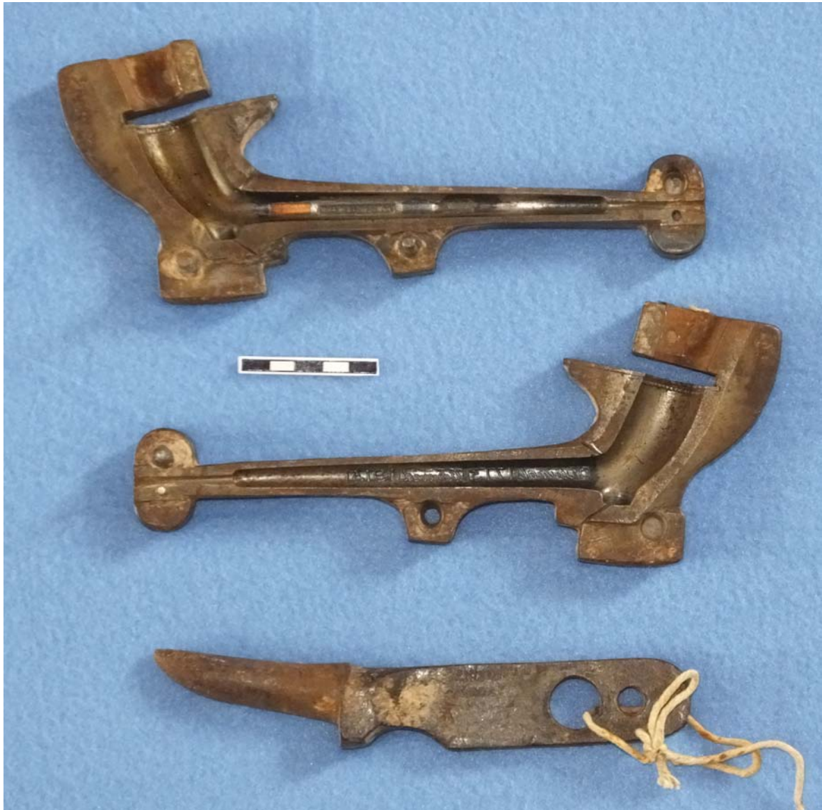
Cast-iron pipe mould comprising two halves to produce the bowl shape (top and middle) and a third part, the stopper (bottom), to form the bowl cavity (Pollock Collection in the National Pipe Archive). Photo D. A. Higgins.
